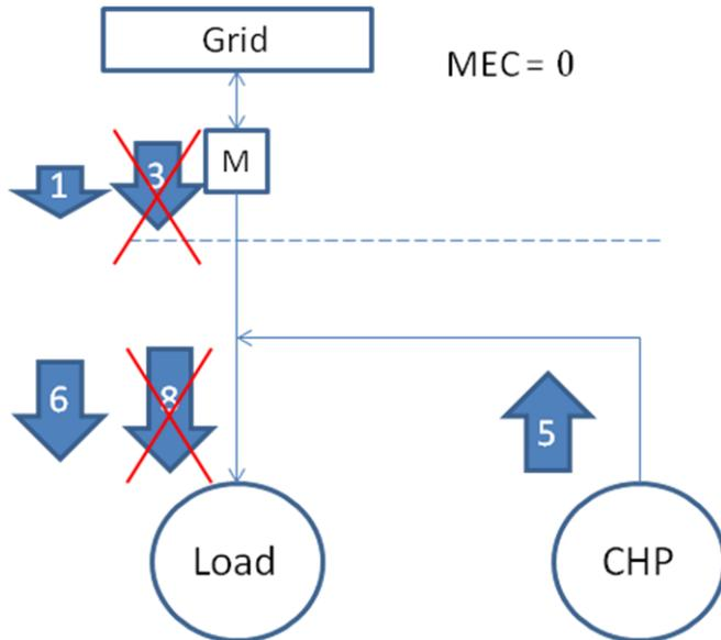
Figure 2 Import only DSU delivering 2MW load reduction
