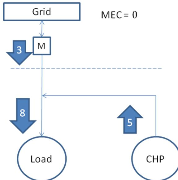
Figure 1 Import only DSU with 8MW load, 5MW CHP and grid demand 3MW
