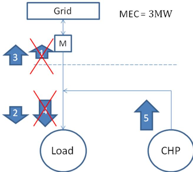
Figure 4 DSU with MEC 3MW offering 2MW load reduction to the system
