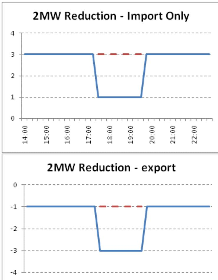
Figure 8 Load Reduction Profile for site with MEC = 0 and MEC = 3MW
