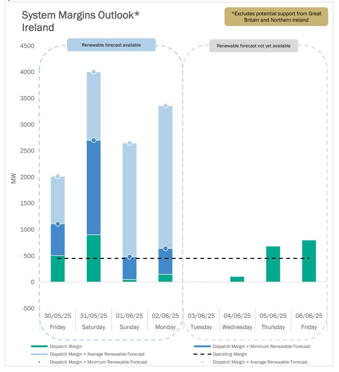
When a negative dispatch margin coincides with a low renewable generation forecast, the net renewable generation value may appear below the zero axis (low forecast: •, average forecast: •). It should be noted that the Daily Dispatch Margin and renewable generation forecast are highly variable. The outlook is based on estimates and is therefore subject to rapid changes.
