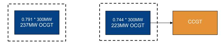
An identical OCGT would "lose" 14MW de-rated capacity when its output is used to feed a separate CCGT component
